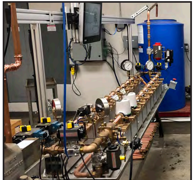
Indianapolis Test Benches can be manufactured to test up to twenty-four 5/8" or 5/8" x 3/4" meters in series.
