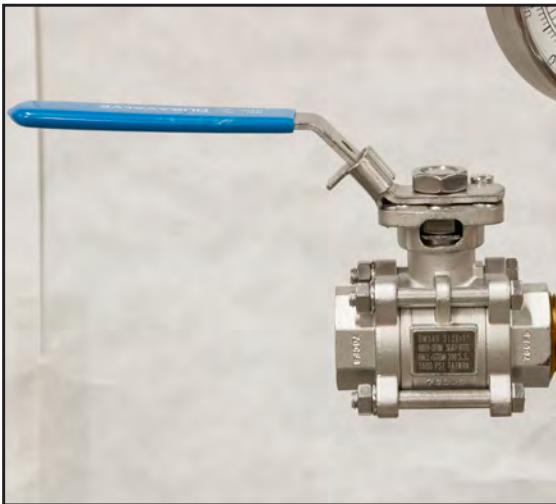
Figure 8 - Bench Inlet Ball Valve (shown in the open position)
