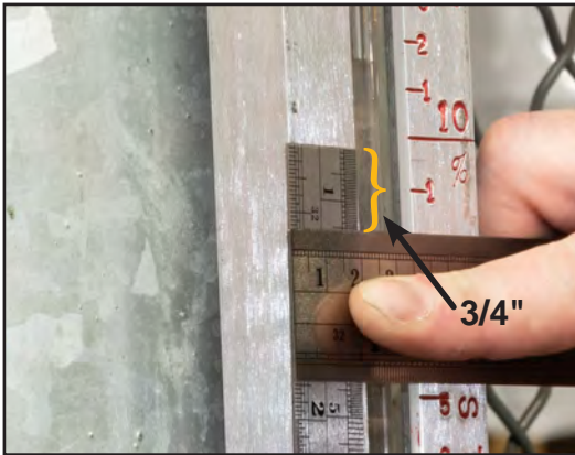
Figure 13 - Example: offset over-run = 3/4"
