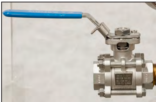
Figure 6 - Bench Inlet Ball Valve (shown in open position)
