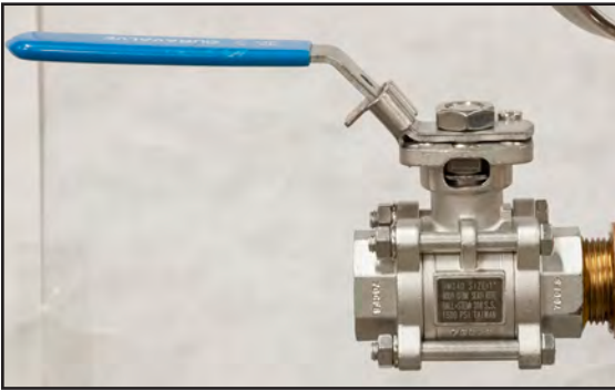
Figure 10 - Bench Inlet Ball Valve (shown in open position)
