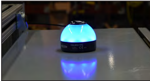
Figure 21 - Blue indicator light on top of the power cabinet indicating attention needed to continue
