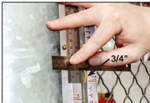
Figure 12 - Example: water over-run = 3/4"
