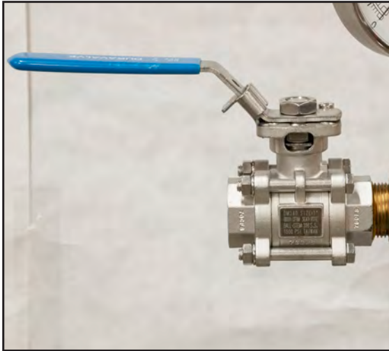
Figure 15 - Bench Inlet Ball Valve (shown in the open position)
