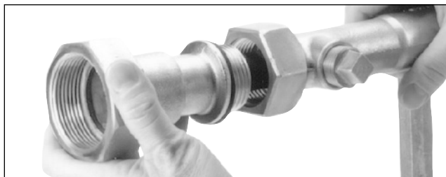
Fig. 2 Select the proper Drilling Machine Adapter and attach it to the Drilling Machine.
