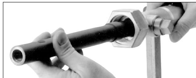
Fig. 1 Insert the Boring Bar into the Drilling Machine.
