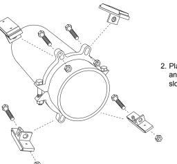
Place the runner on the restraint ring ear and slide the hex head bolt through the slot. Tighten the hex nut securely.
