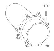
Assemble UFR1300 restraint ring onto pipe, tighten clamping bolts evenly to 200 ft-lbs.
