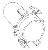
3. Assembled support for Pipe Barrel should appear as shown.
