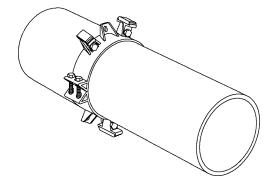
3. Assembled support for Pipe Barrel should appear as shown.
