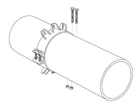
Assemble restraint ring onto pipe. Tighten clamping bolts in an alternating manner (keep gap between restrainer halves even on both sides) to the recommended torque shown on the restrainer.
