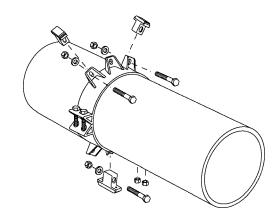
Place the runner on the restraint ring ear and slide the hex bolt through the slot. Place a washer on the bolt and tighten with the nut against it.
