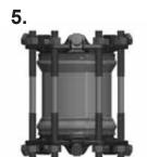
**5.** Loosely assemble a nut on the other end of each restraint rod.
