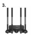
3. Assemble a nut on one end of each restraint rod to approximately two nut widths. Install the restraint rods through one restraint gland with the SO-EZ gasket facing inside the assembly. Stand the assembly on a flat surface with nut side down.
