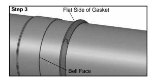
**Step 3.** Lubricate the gasket for best results. Install the gasket around the pipe and lock the ends together. The flat side of the gasket should be positioned against the bell face.
