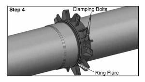
**Step 4.** Loosely assemble (do not tighten the bolts) two ring sections on the spigot side of the pipe with the 1/2" clampling nuts & bolts provided. The flare side of the assembled ring should face the tapered side of the gasket. Assemble the other two ring sections together on the bell side in the same manner.
