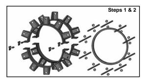
**Step 1.** Check to ensure you have the proper size FBC bell joint leak clamp for your pipe.
