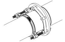
Insert the extra long T-Bolts provided with the Series 1300-P and install one nut each between the gland and clamping ring as shown.
