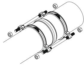
Insert all provided connecting rods and nuts as shown and tighten nuts behind restrainers. Do not over-tighten retaining nuts.
