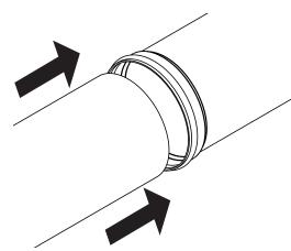
1. Assemble spigot pipe end to bell using standard procedure.
