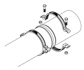
Assemble Series 1390-P clamping rings onto spigot pipe and just behind bell end as shown (use restraining rods as a guide to position and align restrainers) and tighten bolts and nuts evenly to the minimum recommended torque of 100 ft-lbs. A torque wrench is required to ensure proper torque.
