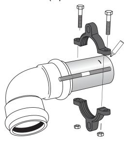
1. Complete the fitting and pipe connection according to the manufacturers' instructions. Install Series 1309 split restraint ring on the spigot end of the pipe. (Use connecting rod as a guide to position split restraint ring as shown above. Mark a line on the pipe approximately 1" shorter than the rod length.) Tighten clamping bolts evenly at least to the minimum recommended torque in the table below. A torque wrench is highly recommended and required to ensure proper torque.
