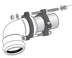
3. Insert extra long rods (provided) through bolt holes on the restrainer and through bolt holes on back-up ring. Place washers against restraint ring and back-up ring ears.
