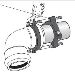
4. Tighten nuts behind back-up ring and restrainer. (Hand tight retaining nuts, then one revolution...do not over-tighten).
