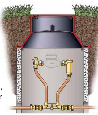
hat shape also provides ground insulation where the cover rests on the pit tile.
