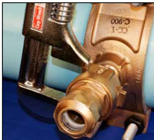
A smooth jaw wrench will fully and properly engage the wrench flats on a valve body or fitting.
