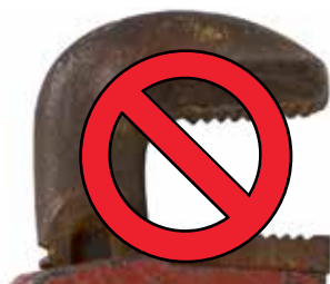
The teeth of a traditional pipe wrench are made for pipe, not brass fittings.
