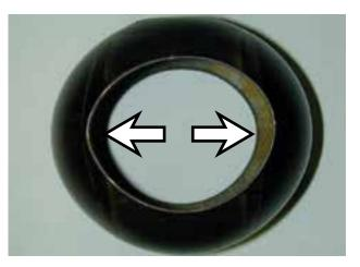
Valve is hard to operate. Ball distortion results from freezing.
