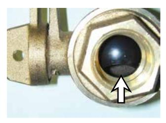
Valve appears to be closed but allows water flow. The ball valve is not fully closed when the tee-head is in a fully closed position.
