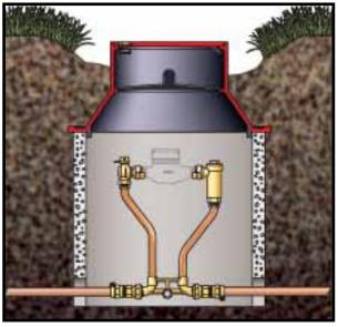
This illustration shows the lid not level with the ground. Voids around the lid should be filled. This protects the cover from damage and pedestrians from possible injury.
