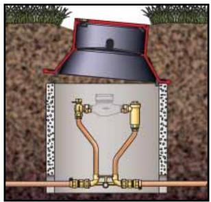
This illustration shows that the cover's frame has shifted and exposed the pit to the surrounding earth. A pit in this condition is in need of immediate repair.
