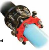
Looking for an easy way to convert a plain end pipe to a restrained flange connection? Look to the Ford Restrained Flange Adapter. Designed with the UFR1400 or UFR1500 restraints *AND* the SO-EZ gasket, these restrained adapters provide a true stab-fit. The restraint gland is furnished with actuating screws designed to twist off at the correct installation torque.
