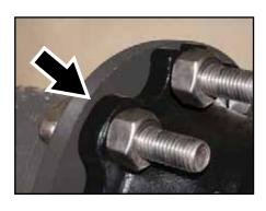
Flange end has two closed starter lugs. This allows the adapter to remain in position while assembling the remaining flange bolts.
