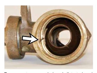
Frozen water expanded and distorted and split the valve body. The valve ball also sustained some distortion.
