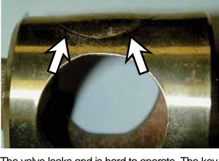
The valve leaks and is hard to operate. The key is bulged from the expansion of frozen water. The key was in the closed position when frozen.
