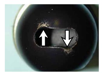
Valve is hard to operate. Ball distortion results from attempting to operate the valve while frozen.
