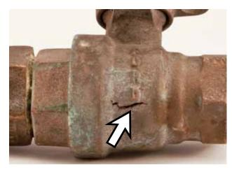
Valve body is split because it was not installed at the proper depth. Frozen water expanded and ruptured the valve body wall.
