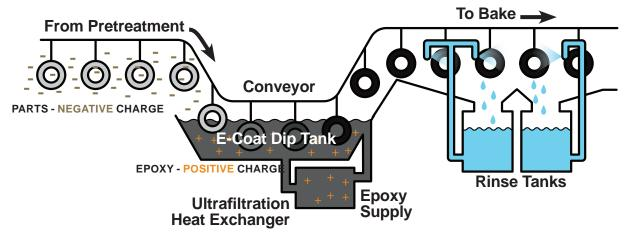
3. PROCESS COMPLETION - Once fully covered, the part is cleaned to remove excess epoxy and then oven-cured to transform the epoxy particles into a uniform protective shell. E-Coat's high quality black finish is resistant to damage from impact, abrasion and corrosion.
