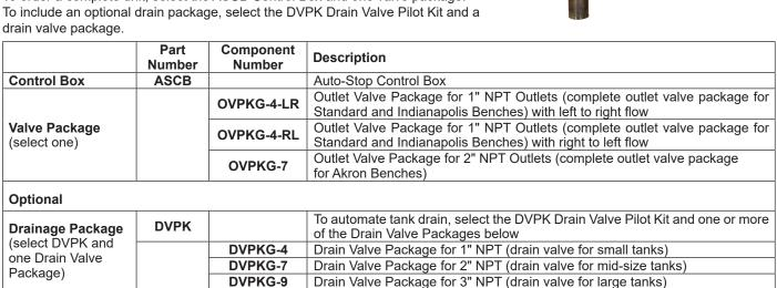
Note: A small compressor (not included) capable of 90 to 100 psi is required to operate the valves on the Auto-Stop.
