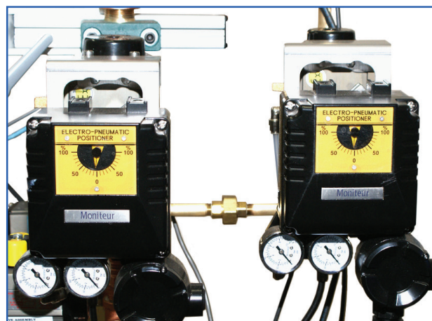
Outlet assembly with pneumatically powered flow control valves
