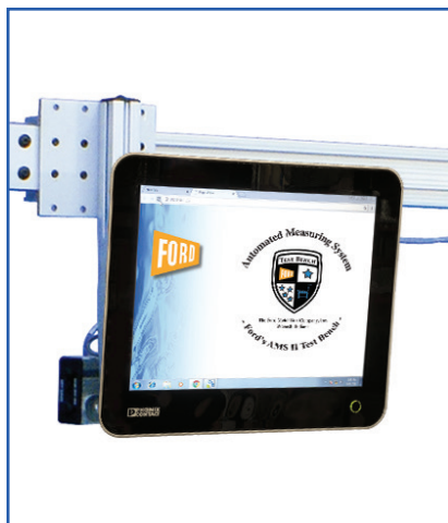
Waterproof touch-screen PC monitor attaches directly to the test bench for easy access
