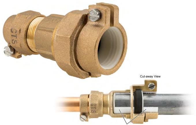
Permanently installed plastic gripper ring and sleeve liner prevent direct contact between lead pipe material and other metallic water system components
