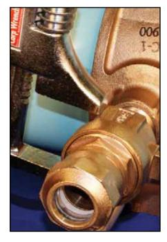
Ford Meter Box recommends the use of tightly engaged, smooth-jawed wrenches because they do not distort fittings or valves during installation. The smooth jaws of the RCORP Wrench (or similar RIGID smooth-jawed wrenches) are strong yet gentle on valves and fittings. A coarse adjustment thread and large thumbscrew provide quick and easy movement for the numerous size changes encountered on the job. For more information, contact Ford Meter Box or your local Ford distributor.
