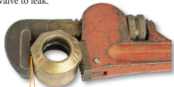
Above is a view of non-parallel pipe wrench jaws improperly engaging parallel wrench flats.
