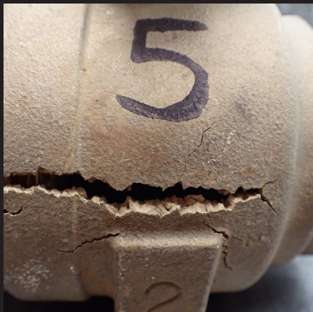
Images above capture the impact of freezing water inside a brass valve. From left to right: cracked valve body, oblong ball, and expanded plug valve key.
