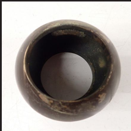
Images above capture the impact of freezing water inside a brass valve. From left to right: cracked valve body, oblong ball, and expanded plug valve key.
