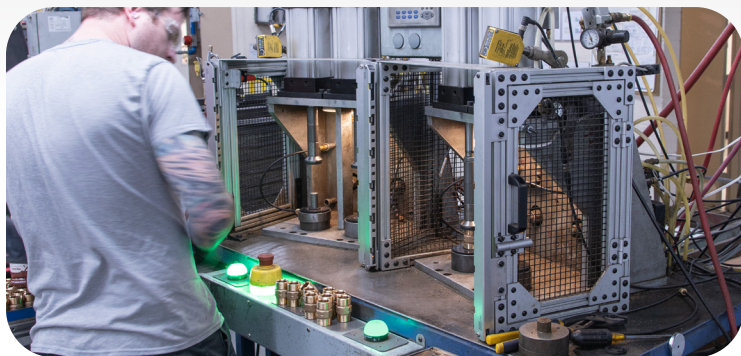
Large air testing machines are testing a variety of angle valves, check and key valves, and couplings, to ensure that each part does not leak.
