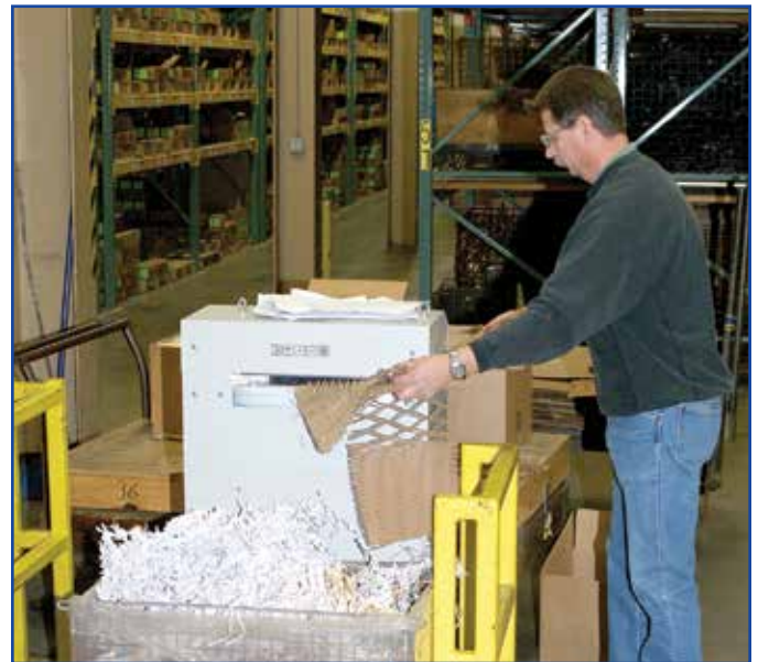
The PacMaster™ perforates scrap paper and cardboard for use as packing material.
