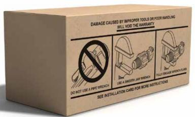
Waterworks brass contains a high percentage of copper and is relatively soft. It has proven to be extremely durable once installed; however, it must be handled with care during installation and backfilling. The improper use of a wrench will distort a valve or fitting resulting in possible leakage. Ford Meter Box recommends the use of a smooth jaw wrench that fits snug across the wrench flats of the valve body to ensure a tight connection without distorting the brass valve body.
