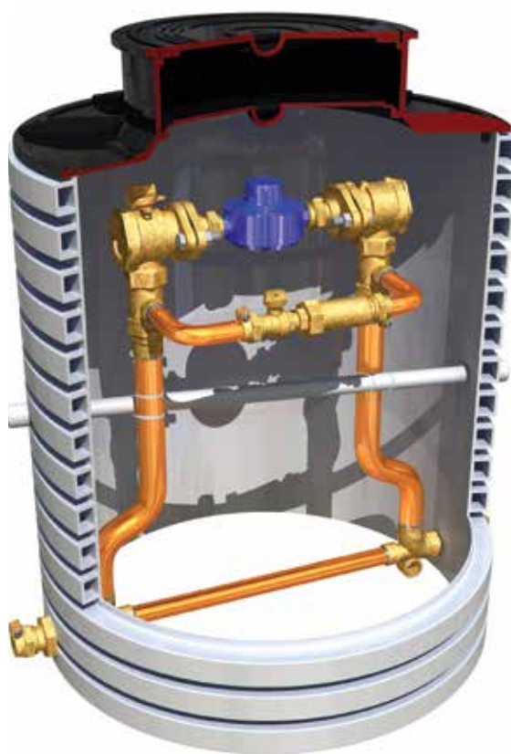
A 2" Plastic Pit Setter fitted with two A47 meter adapters change a 2" flanged meter setting to accommodate a 1" meter
