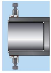
for easy insertion while preventing over-insertion. Just slide the insert into the pipe or tubing before connecting the pipe to a compression fitting or restraint. Available in DIPS or IPS sizes, simply measure the pipe or tubing ID to ensure the correct size is used.
