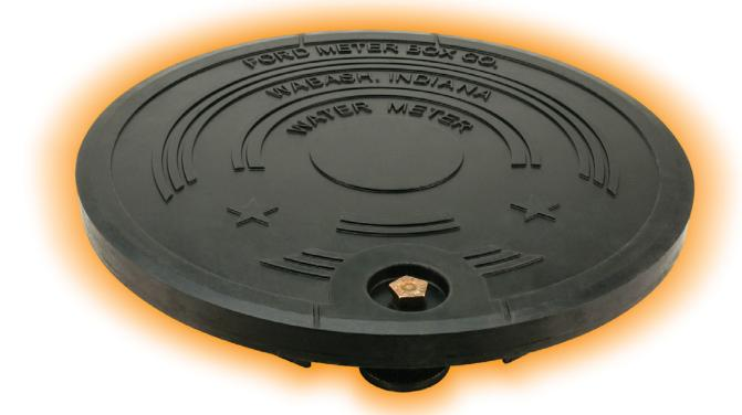
For heavy duty lid applications that require low AMR signal interference, Ford offers two new coil pit lids. With an H-20 rating meeting 40,000 pound proof load for traffic requirements, these lids for 15" and 18" tile are durable and UV resistant.
