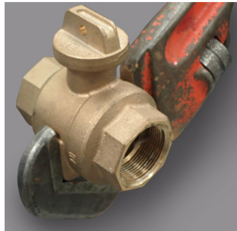
The photo above shows a smooth jaw wrench properly engaging the wrench flats on a valve.
