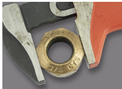
This photo shows proper wrench position on a compression nut.
