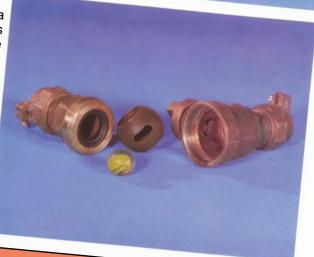
Top: This photo of the valve partially disassembled shows the marble lodged inside the ball. The marble, once in the Ball Valve, could not exit.
