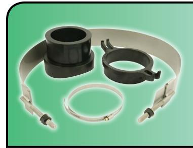
Ford Sewer Saddles are available in a wide range of connection and pipe sizes. With a 304 stainless steel band that adjusts to fit an array of pipe sizes and a Buna-N gasket to ensure a secure seal, the Ford Sewer Saddle is ideal for non-potable water applications. A quick and simple installation will ensure a secure connection with up to 7 psi working pressure in no time.
