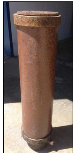
This original Ford meter box recently unearthed in Hartford City, Indiana, remains functional after more than 100 years.
