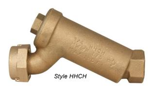
Ford offers two styles of in-line accessible cartridge dual check valves, angle and straight. The Ford® Cartridge Dual Check Valve (Style HHCH) and Angle Cartridge Dual Check Valve (Style HHCA) allow inline access to the internal components of the check valve. A removable O-ring sealed cap at the top of the valve allows access to the dual check components for maintenance, inspection or replacement. Ford Meter Box cartridge dual check valves meet or exceed all requirements of ASSE Standard 1024.
