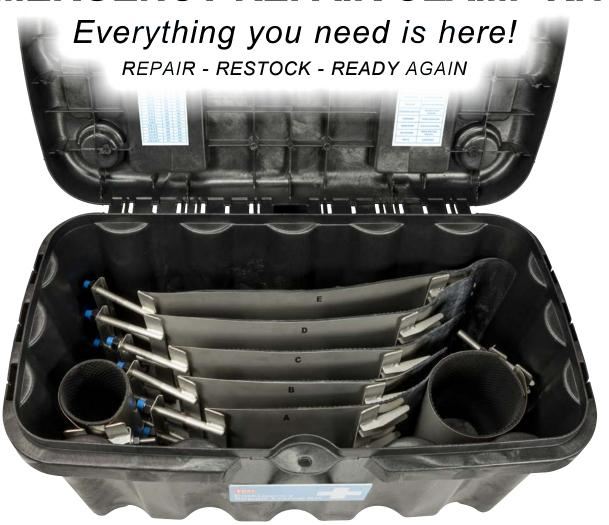
The Ford Emergency Repair Clamp Kit contains stainless steel bands that combine in various configurations to provide quick and reliable pipe repair for 4.50" to 30.75" pipe diameters. The kit's components are neatly arranged in a durable and restockable case that can be stored in the shop or truck.
