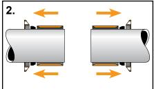
2. Slide the two end rings, end ring gaskets and sleeves over the exposed ends of the pipes as shown.
