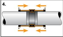
4. Slide the end rings, end ring gaskets and sleeves toward the cut-in sleeve.
