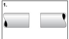
1. Clean each end of the pipe to ensure a watertight seal.
