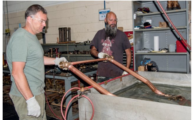
Each setter is tested for leaks before installation in a pit.
