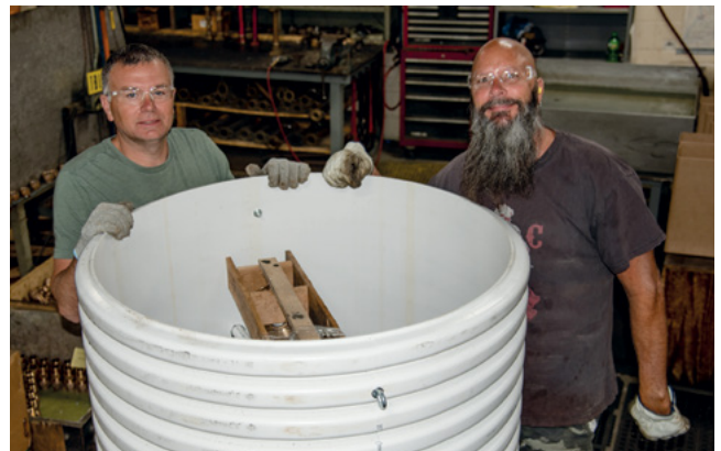
The setter is braced to prevent movement during shipment.
