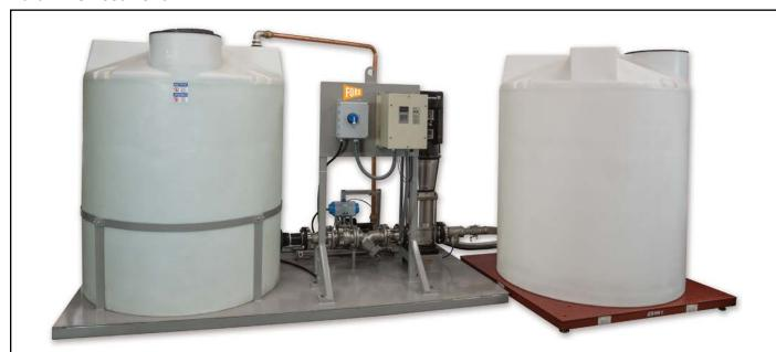
Traditional water meter testing sends all the water down the drain after the tests are run. Ford's recirculating system eliminates this lost water by constantly recycling test bench water. The two tank system provides a constant and steady flow for accurate tests.
