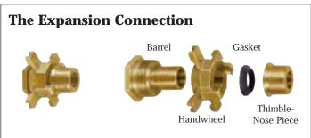
Handwheel Nose Piece made it possible to install and remove a meter in a setting conveniently by hand. It replaced the awkward wedge device and revolutionized water meter settings.
