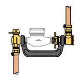
operated. Angle yoke valves and ells can be rotated to connect to piping from any direction.
