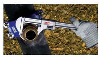
Major brass fittings manufacturers recommend RCORP when tightening corp stops, either into the pipe or tapping saddle, or tightening service line connections on any waterworks brass valve or fitting.
