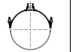
12" 202B DOUBLE STRAP BRASS SADDLES FOR DUCTILE IRON PIPE WITH 1-1/4" FIP OUTLET,
