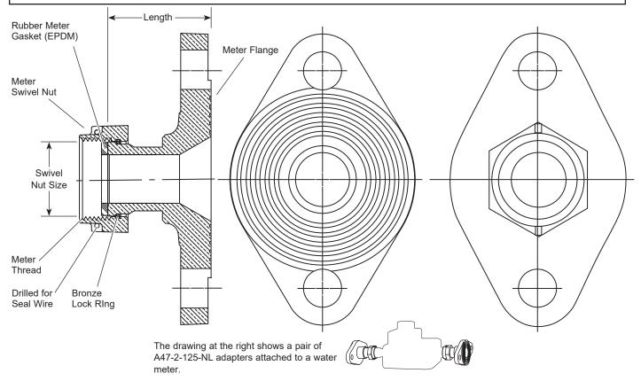
One pair of this adapter converts the overall lay length from 10-3/4" to 15-1/4".
