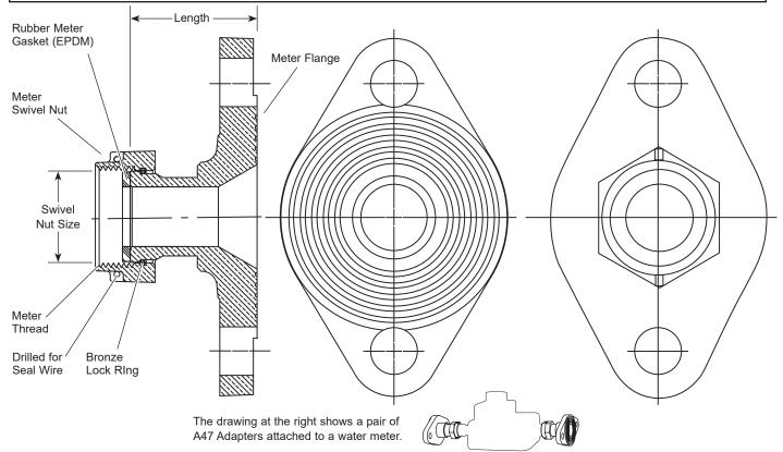
One pair of the A46-NL converts the overall lay length from 10-3/4" to 13". One pair of the A47-NL converts the overall lay length from 10-3/4" to 17".no
