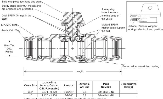
Note: Ford recommends using insert stiffeners with plastic pipe or tubing.
