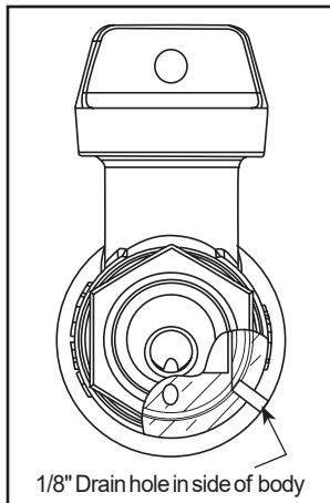
1/8" Drain hole in side of body
