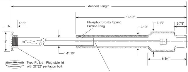
Steel Stationary Rod with Ductile Iron Tee Head Socket and Brass Cotter Pin
