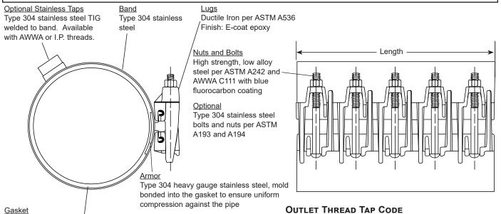
Gridded Virgin SBR compounded for water service, per ASTM D2000. NBR (Buna-N) is available.
