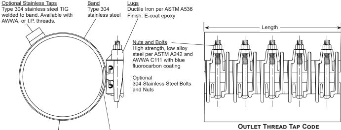
Gasket Gridded SBR rubber compounded for water service, per ASTM D2000.
