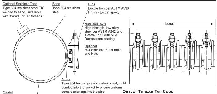
Gridded NBR (Buna-N) compounded for water service, per ASTM D2000.
