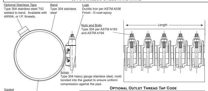
Gridded Virgin SBR compounded for water service per ASTM D2000. NBR (Buna-N) and EPDM are optional.
